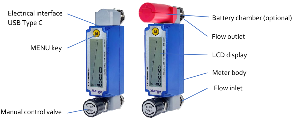
Figure 3.1: MF6600 parts description
