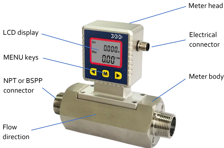
Figure 3.1: MF5900 parts description
